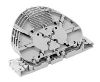
FIST<sup>TM</sup> Splice Sub-assembly kit with 4 trays, each for holding up to 12 primary or 4 secondary coated fibers, with Heat Shrink type splice holder
